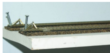
Bumpers are securely anchored to keep locomotives from falling off the end.
