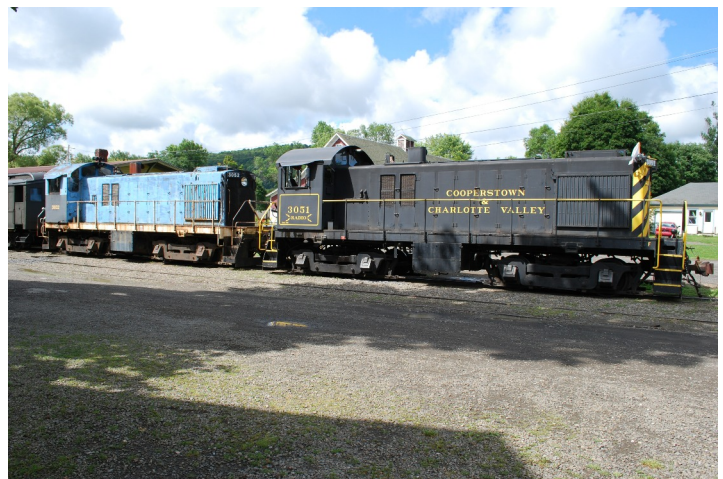
Photo 3: CCV MLW S4 switchers
