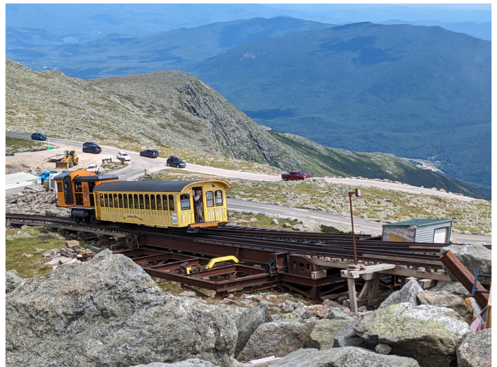
One of the diesels pushes a car onto the upper switch. These sliding switches are very impressive and would be quite a thing to model.
